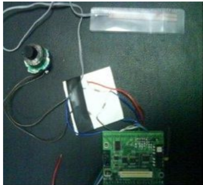
Fig 1 prototype of real-time warning system using WSN
